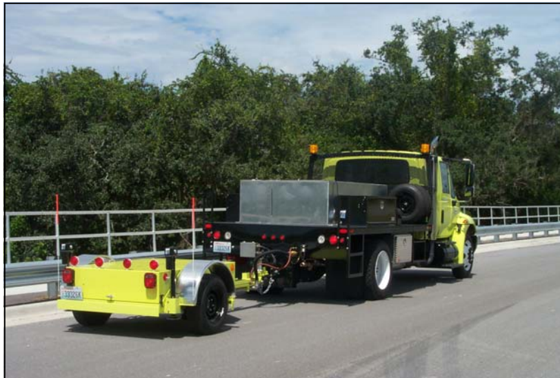
Certified by TTI as an ASTM E274 Friction Tester
